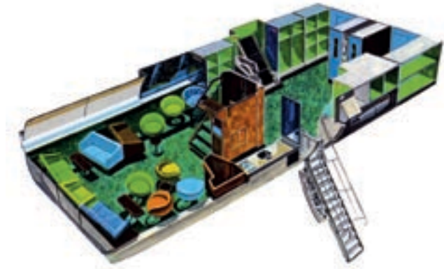
The lower-deck carry-on luggage area and lounge with an integral staircase located on the left-hand side of the aircraft.
